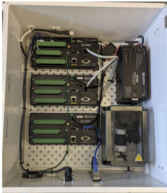
Figure 2. View of the interior of one of the identical enclosures housing PAR instruments mounted on S13 and S14 towers. The uppermost datalogger is dedicated to the PAR instrument, and is wired to three PAR sensor connectors shown at the bottom of the image. The other two loggers in the enclosure share the power supply and are used in the WXT520/530 meteorological instrument system (METWXT) and infrared thermometer (IRT) instruments co-located on each of the towers.
