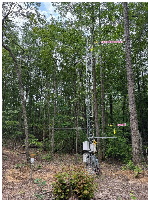
Figure 4. Side view of S13 tower showing position of PAR sensor booms at 2 m and 8 m. The 8 m boom extends away from the camera.
