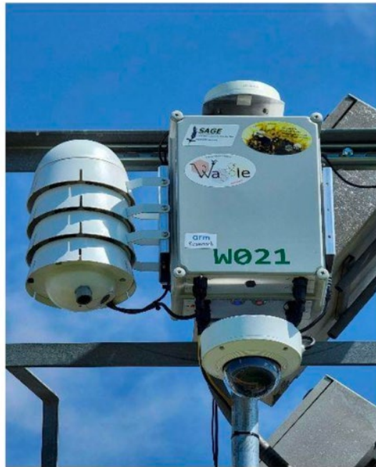
Figure 1. Waggle node at the U.S. Department of Energy (DOE) Atmospheric Radiation Measurement (ARM) user facility’s Southern Great Plains (SGP) observatory featuring a sky-facing and a ground camera with Stevenson shield, serving as an edge computing node for real-time atmospheric data collection and analysis.
