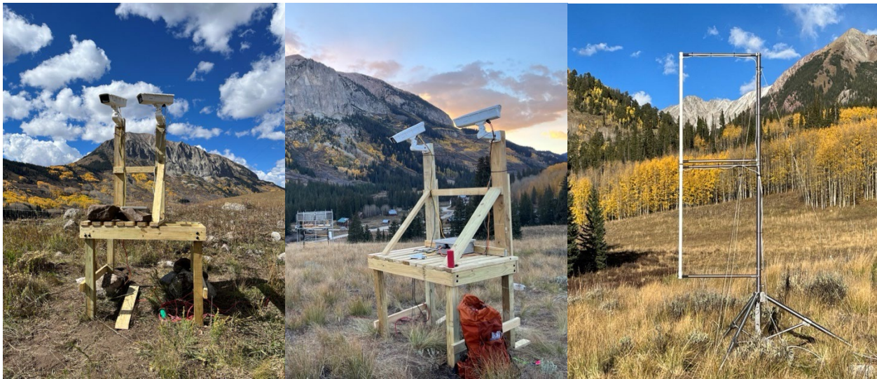
Figure 1. Instruments deployed during SAIL-TOBS. Left: OSCRE at Kettle Ponds. Middle: OSCRE at AMF2 in Gothic. Right: FlowCapt FC4s at AMF2.
