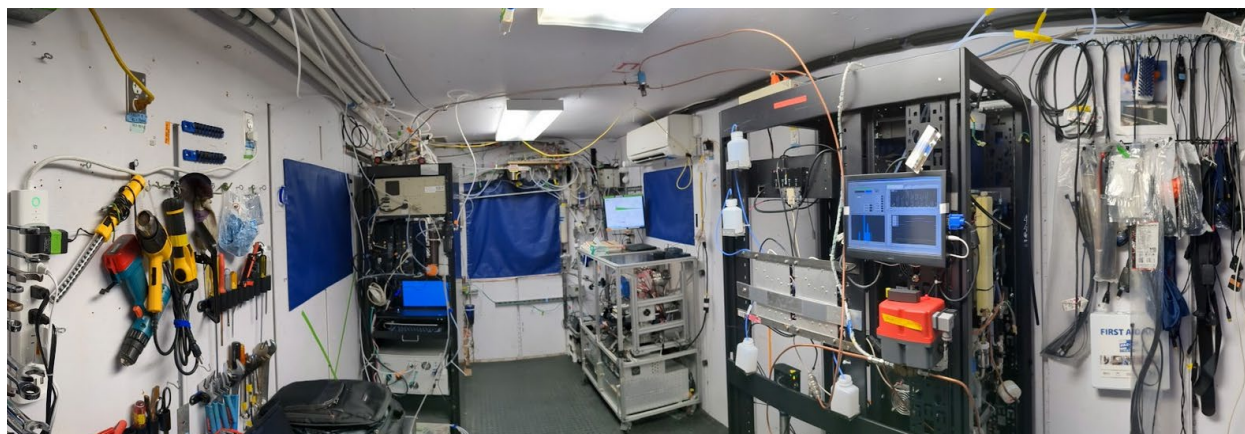
Figure 1. Interior of the trailer. The denuded/undenuded CCN rack is to the right.
