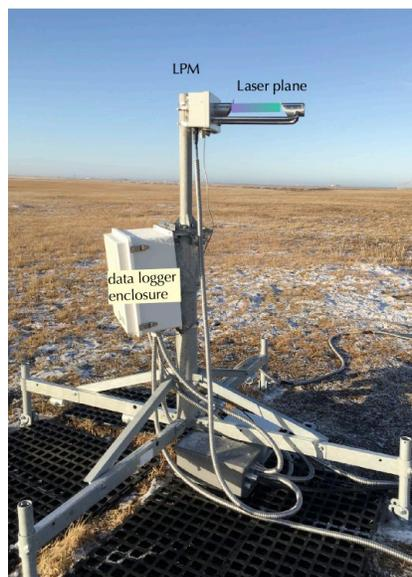
**Figure 27.** The C1 unshielded LPM. (E10 operated at the C1 site).
