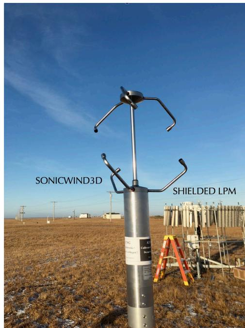
**Figure 15.** Thies-Clima three-dimensional sonic anemometer (SONICWIND3D). In the background is the double Alter shield surrounding the LPM.
