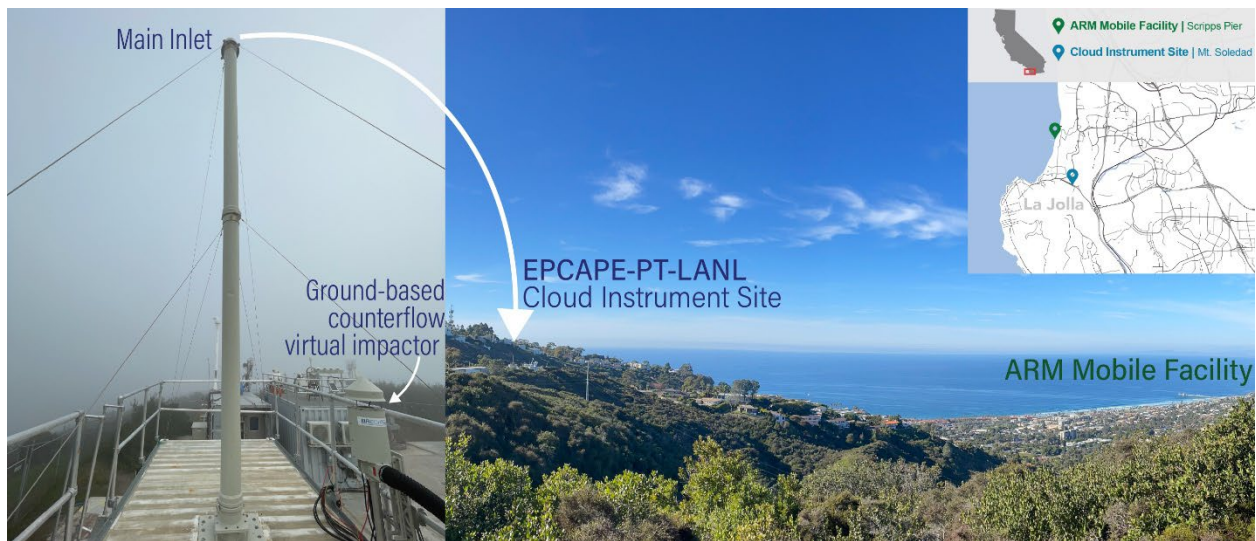
Figure 1. Left: main inlet and ground-based counterflow virtual impactor (GCVI) with picture taken during cloud sampling. Right: picture of the EPCAPE-PT-LANL instrument container at the Cloud Instrument Site on Mt. Soledad site with a view towards the Pacific Ocean showing the EPCAPE main site for the ARM Mobile Facility on the Scripps Pier [1].
