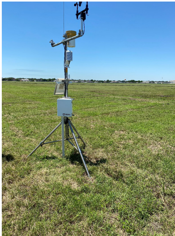
Figure 2. Soil water content monitoring station with additional meteorological monitoring equipment located in La Porte, Texas. Instruments are similar to Figure 2 in part II of this ARM field campaign report, DOE/SC-ARM-23-019.
