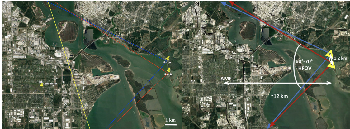
Figure 1. Stereo camera positions with respect to the AMF M1 LaPorte Airport site. The blue/red lines identify the field of view of the cameras “Hou-A” and “Hou-B”, respectively. Clouds > 10 km in depth fit in the field of view of the cameras starting at the yellow line.
