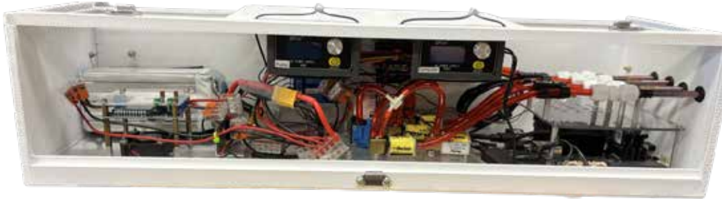
Figure 2. Modular VOC sampler with top and side access panels open. The unit is capable of collecting up to four samples per flight.
