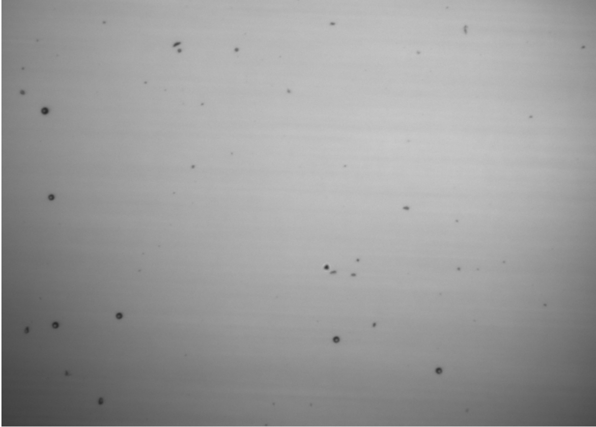
Figure 1. An ngVIPS image from a heavy fog period. The field of view is approximately 3mm across with the larger drops in the lower portion of image being approximately 30 microns in diameter. Some slightly irregular particles are visible in the frame that are likely ice particles. More typically, the particles were similar to the smaller specks in this image, indicating that they were on the order of 5-10 microns.
