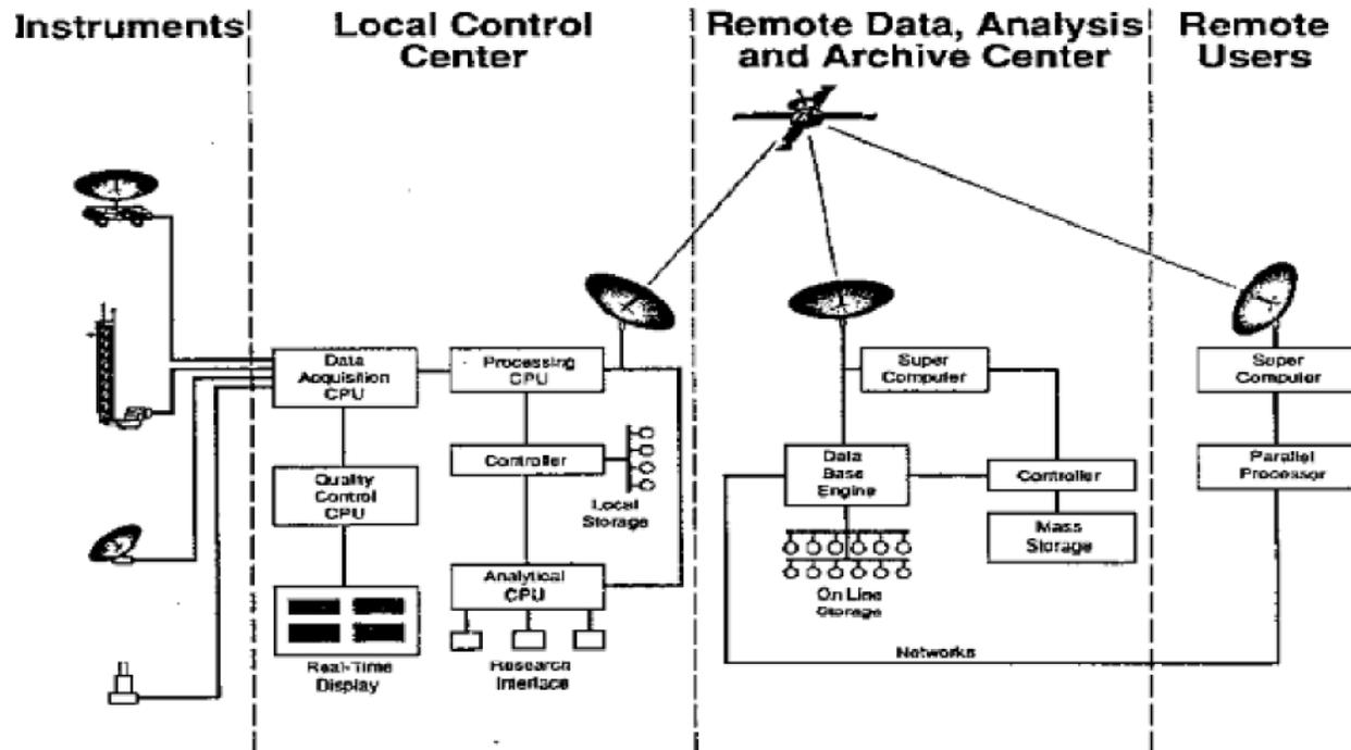
**Figure 18.** Components of the ARM data management system.
