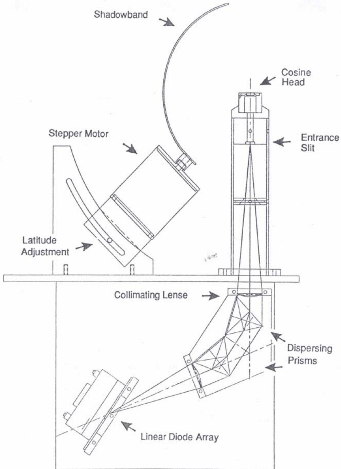
**Figure 23.** The Rotating Shadowband Spectrometer.
