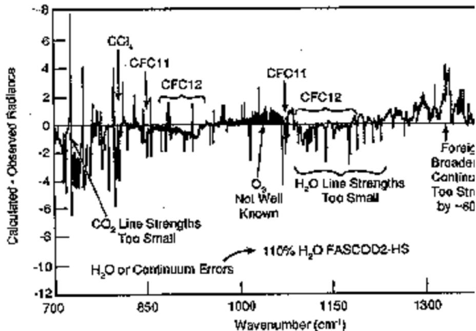
**Figure 6.** The difference between FASCOD2-calculated and HIS-measured radiance spectra found by Dr. William Smith, University of Wisconsin.
