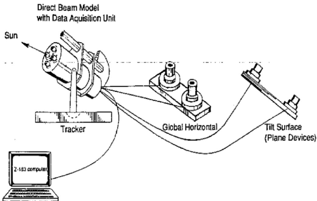
**Figure 16.** The calibration of radiometric instruments often involves the intercomparison of different kinds of sensors using the sun as the calibration source. A fairly common method of calibration involves the use of a tracking radiometer. The system shown here is in use at SERI
