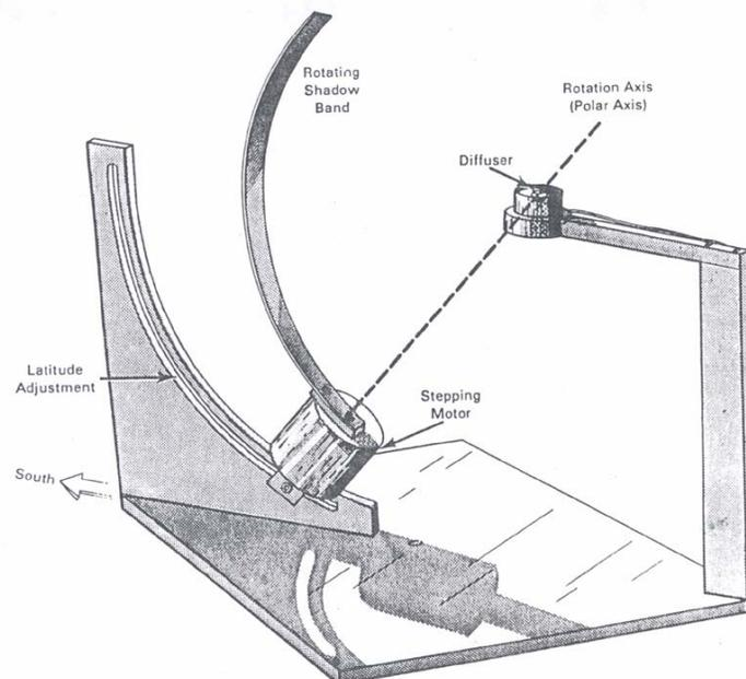
**Figure 22.** The Rotating Shadowband Radiometer.
