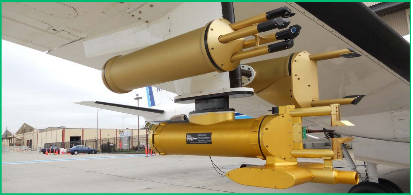
Pylons attached to the underside of ARM aircraft wings carry a variety of instruments that measure cloud and aerosol properties.
