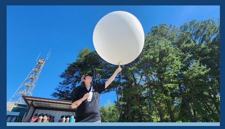
On September 18, 2024, technician Kris Bennefield prepares for a test launch of a balloon-borne radiosonde at the main site of ARM's Bankhead National Forest atmospheric observatory.
