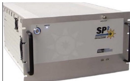
Single Particle Soot Photometer (SP2) Black Carbon
