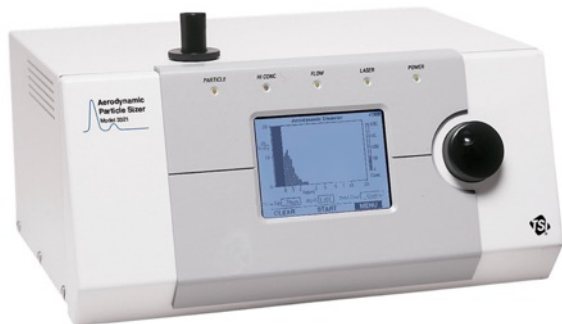
Aerodynamic Particle Sizer (APS) Larger aerosol diameters .5 – 20 \mu\text{m}
