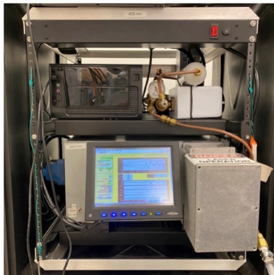
Single-Wavelength Integrated Photoacoustic Nephelometer (IPN; 405, 721, 1047 nm)
