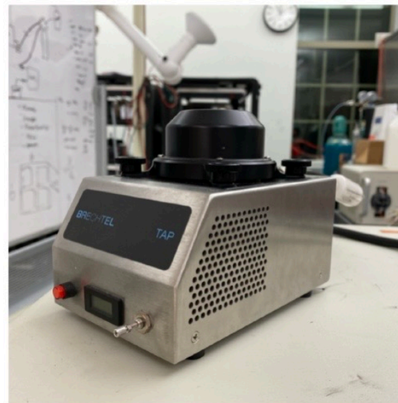
Tricolor Absorption Photometer (TAP; 467, 528, 652 nm)
