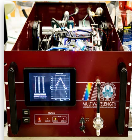
Multi-Wavelength Integrated Photoacoustic Nephelometer (MIPN; 405, 488, 561, 670 nm)
