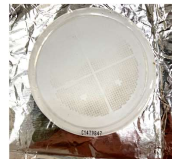
Non-size-selected filter sample for offline chemical analysis. Photo: Vandergrift/EMSL.
