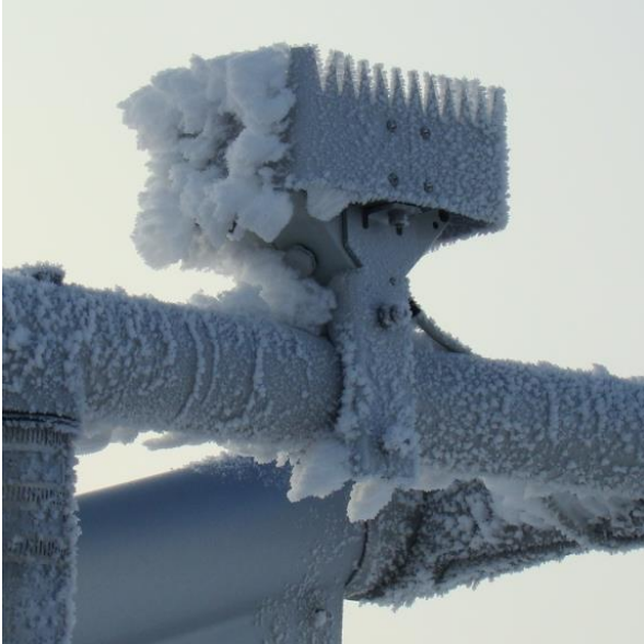
Frost gathers on the all-weather sensor, which measures precipitation amounts and extinction (visibility).
