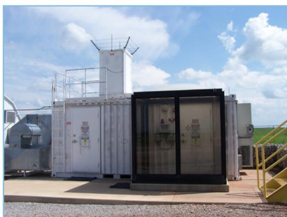
Developed for ARM as the first turn-key operational Raman lidar in the world, the original ARM Raman lidar has operated nearly autonomously at the SGP site since 1996. Recovery Act upgrades include a new laser system, a new beam-expanding telescope for the transmitted beam, and updating the computer operating system and the lidar control software.
